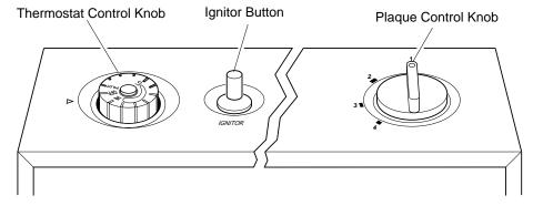
Figure 16 - Thermostat Control Knob In The OFF Position
